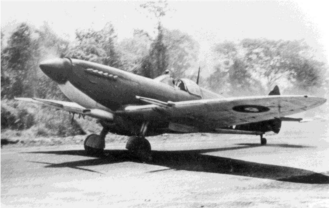
**Forrest Green 54 Sqn RAF Spitfire A58-352 DL-N with slipper tank fitted as per operation.**
